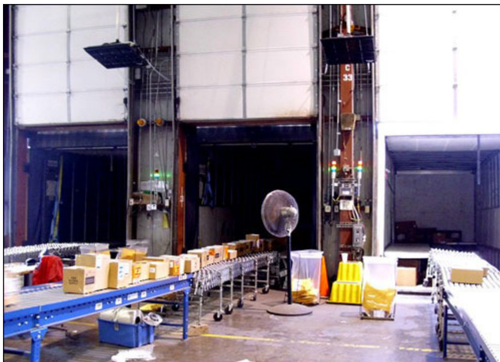
The system issue alerts if boxes or bags are being loaded onto the wrong truck, or if an item falls off a conveyor and is at risk of being misplaced.
